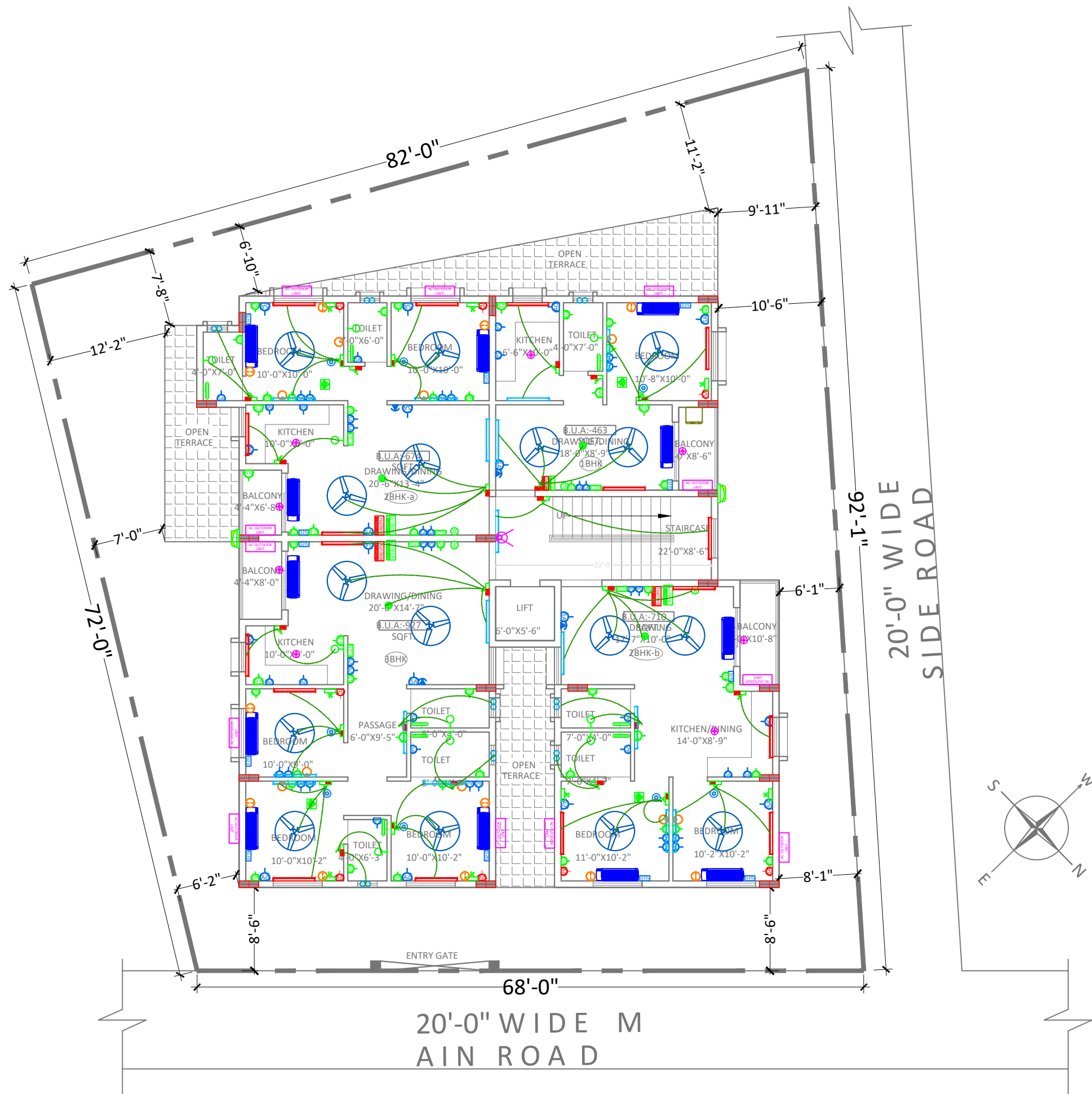
TYPICAL (1to 3rd) FLOOR ELECTRICAL CIRCUIT LAYOUT
