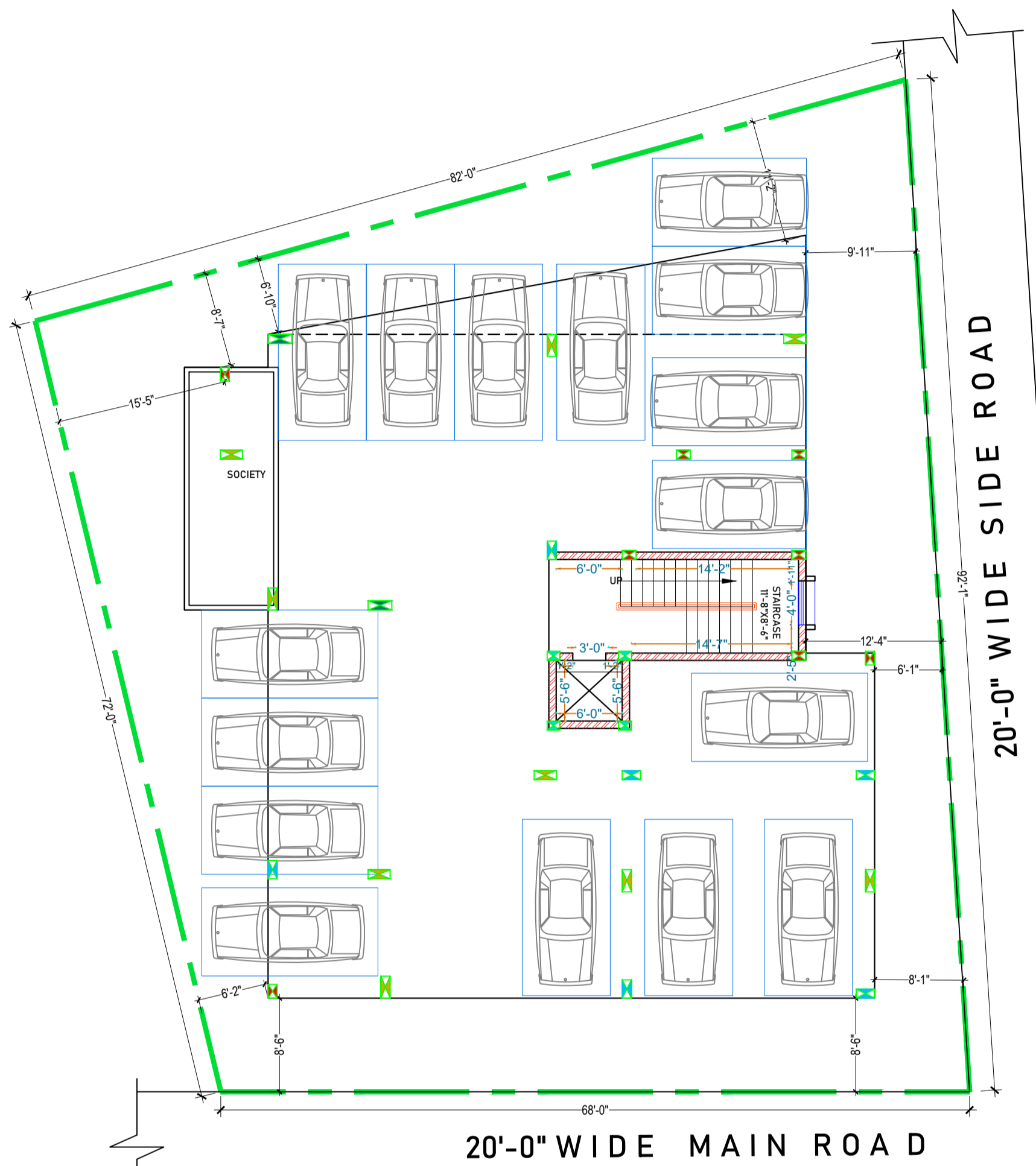
STILT FLOOR AREA STILT ROOF AREA - 3527 SFT
